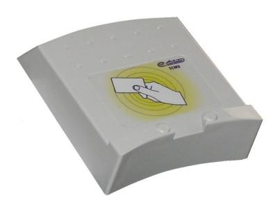
The **Cartadis TCM2** is reader of contactless or proximity cards, compatible with most of the cards on the market in 13.56 Mhz or 125Khz technology. By default, its emulates an USB keyboard and so a driver installation is not required on Windows PCs.
